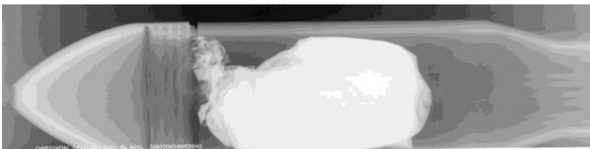
Figure 5.9 An X-ray image showing the contents of a Type 5 munition believed to contain sulphur mustard (source: ARES/confidential).
