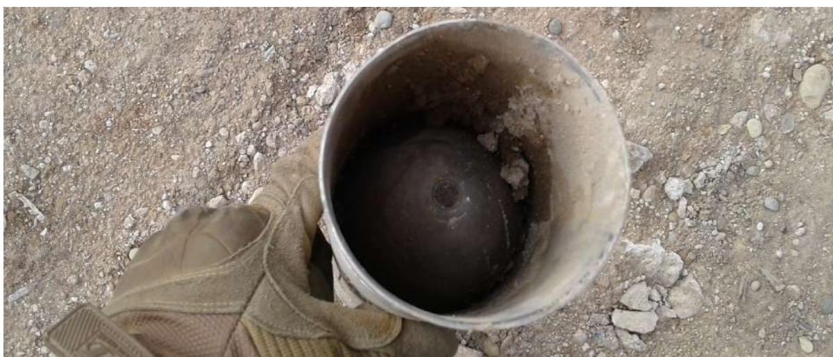
Figure 5.2 A tube (probable recoilless gun barrel) with an unidentified munition with a plastic warhead loaded inside, encountered in Mosul in November 2017 by an EOD team (source: ARES/confidential).
