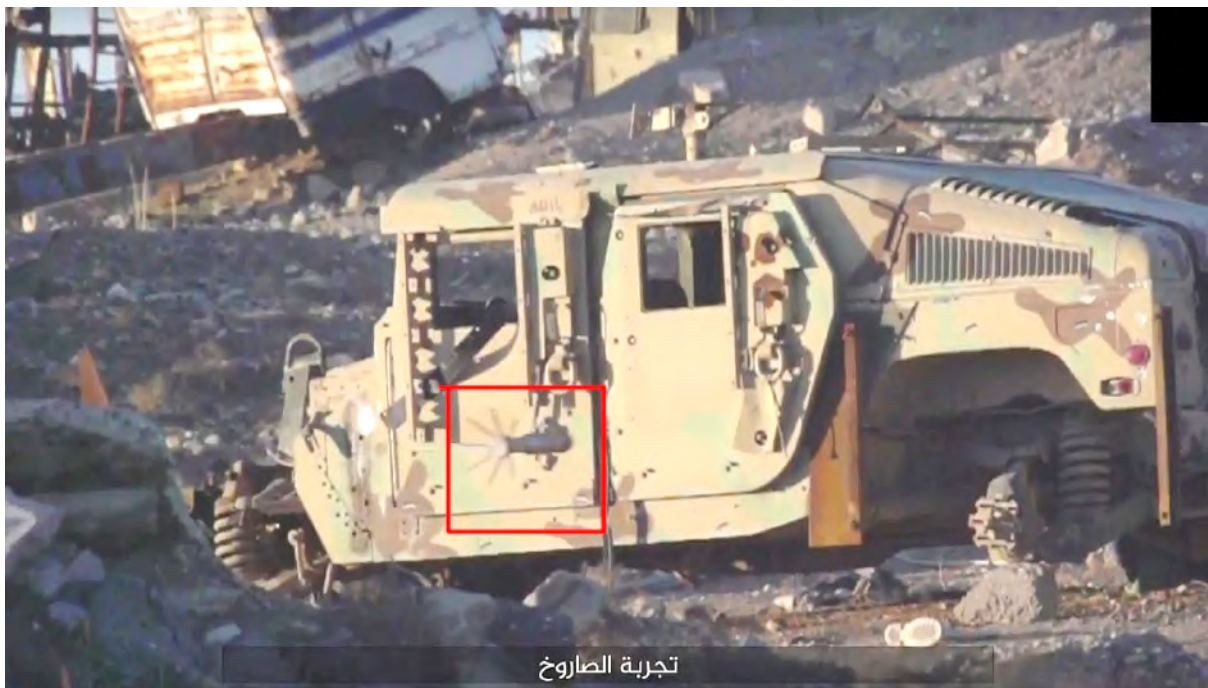
Figure 3.5 An IS Type 4 projectile about to hit a lightly armoured vehicle. The vehicle has no wheels and appears to be a test target (source: IS media via ARES CONMAT database).
