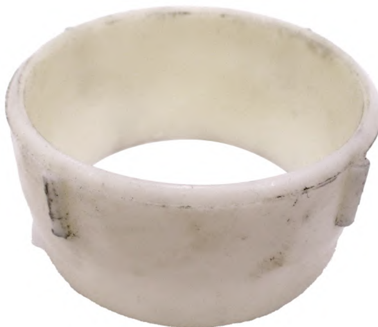
Figure 3.22 The plastic collar (centring ring) which is place around the ogive of the Type 2 and Type 3 projectiles to centre it in the barrel of the recoilless gun (source: Drew Prater).
