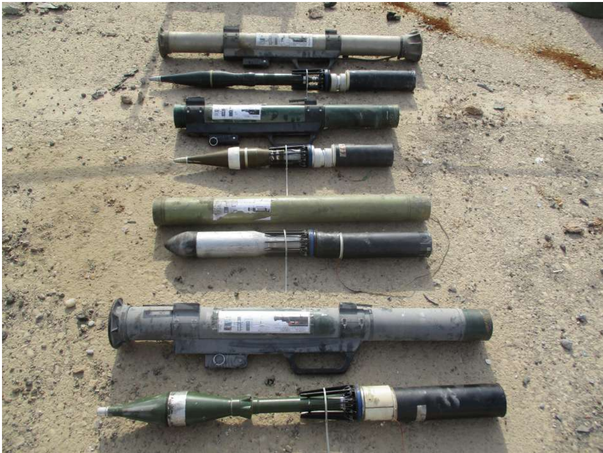
Figure 1.2 The four previously documented Types of IS craft-produced recoilless light guns. From top to bottom: Type 2; Type 3; Type 4; and Type 1 (source: Drew Prater).
