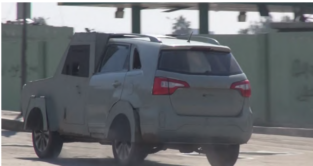
Figure 2.1 A suicide vehicle-borne improvised explosive device used by IS in Mosul, Iraq, in March 2017. Note the armoured forward section of the vehicle (source: IS media via ARES CONMAT Database).
