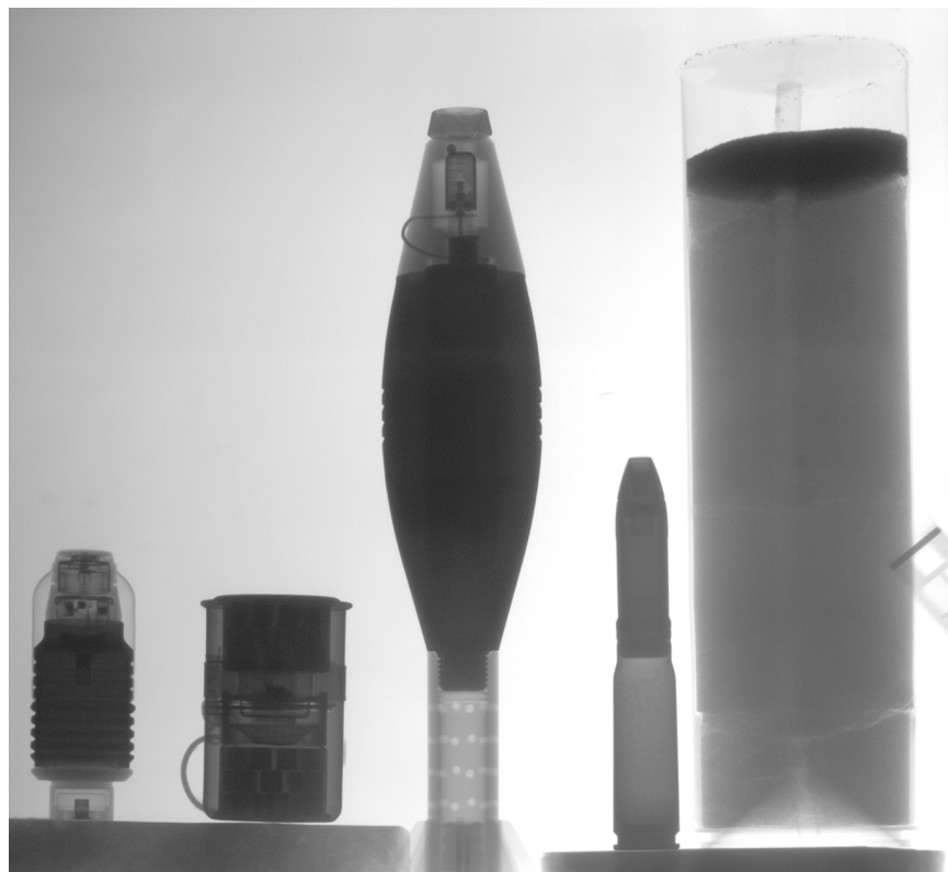
Figure 3.15 Counter mass assemblies in various states of assembly in Mosul, Iraq, in February 2018. These examples contained sand as a counter mass (source: ARES/confidential).
