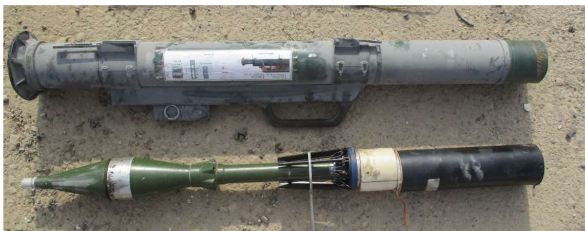
Figure 3.20 The Type 1 ('PG-7V') IS light recoilless gun and its Type 1 munition. Note that what appears to be a silver 'band' on the munition warhead is actually the result of the green paint being abraded from the projectile due to the very tight fit between the PG-7 warhead (~85 mm) and the tube (internal diameter of ~84.5 mm) (source: Drew Prater).
