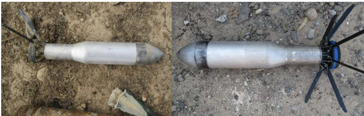
Figure 3.26 Two images of the Type 4 projectile. Note the fully extended fins in the right-hand image (source: Drew Prater).
