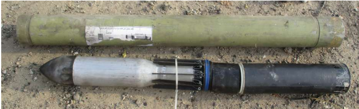
Figure 3.25 The Type 4 (‘Thermobaric’; actually HE) IS light recoilless gun and its Type 4 munition. Note the gripstock assembly is absent from this example (source: Drew Prater).
