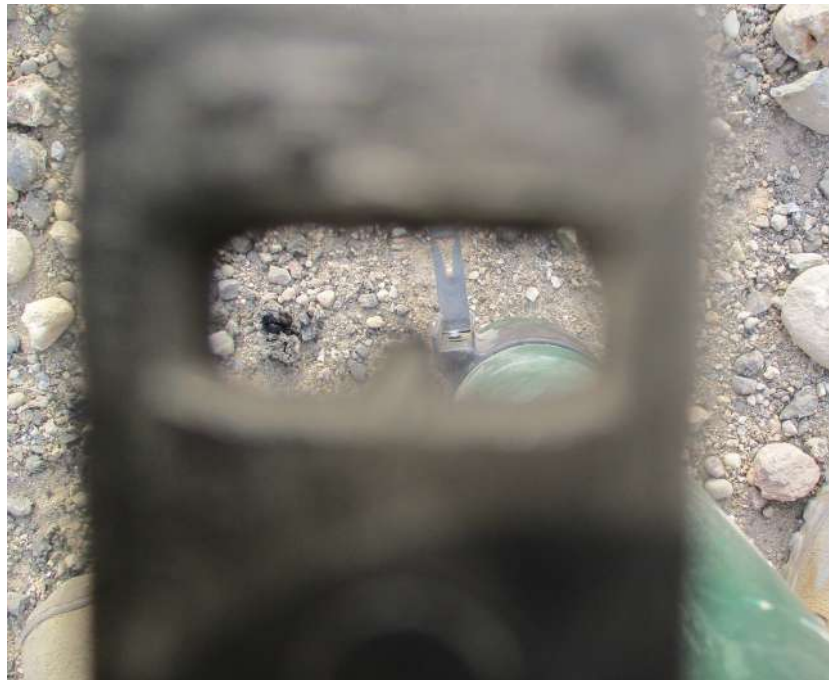
Figure 3.24 The sights lined up on a Type 3 light recoilless gun (source: Drew Prater).
