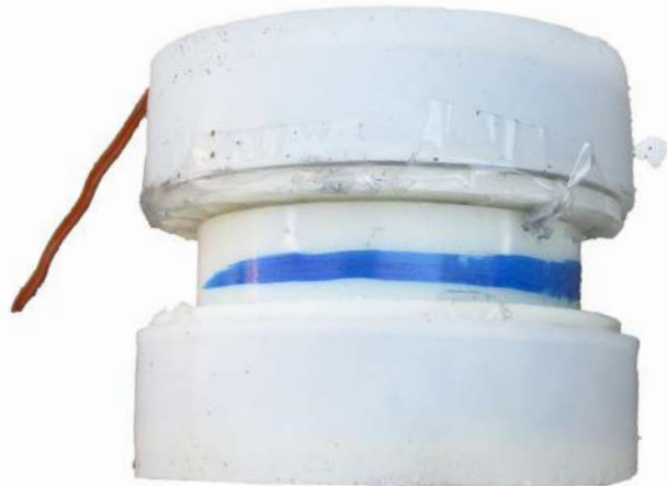
Figure 3.12 The IS propelling/expelling charge, without its outer sleeve, showing the three chambers (source: Drew Prater).
