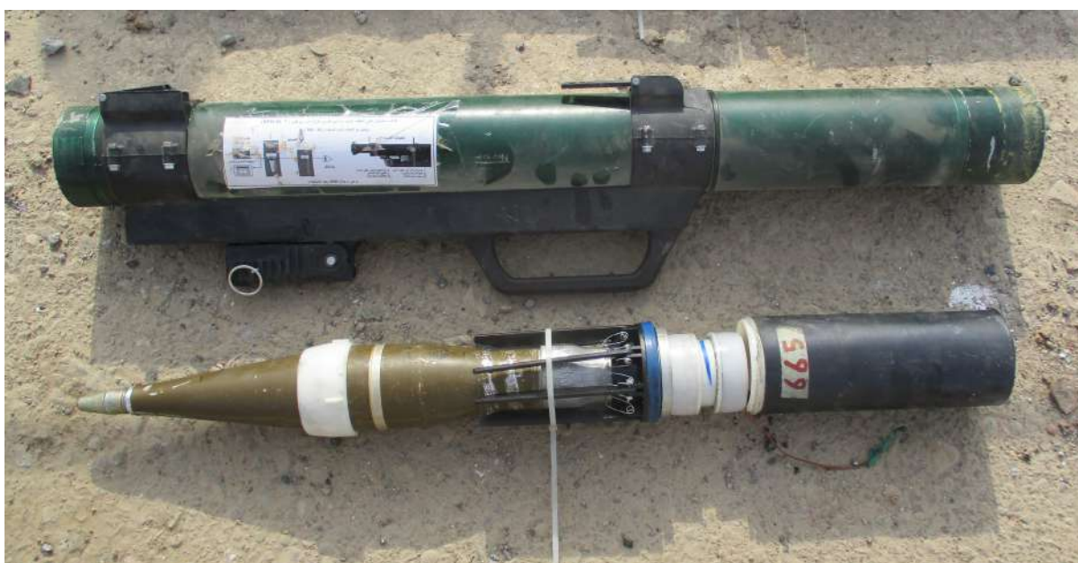
Figure 3.23 The Type 3 ('PG-9 SR') IS light recoilless gun and its Type 3 munition (source: Drew Prater).
