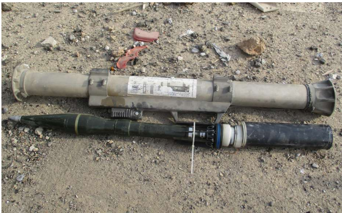
Figure 3.21 The Type 2 ('PG-9 LR') IS light recoilless gun and its Type 2 munition (source: Drew Prater).
