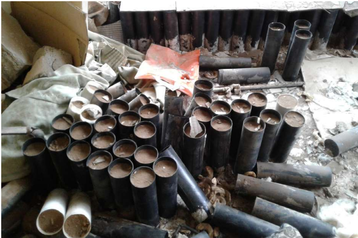
Figure 3.15 Counter mass assemblies in various states of assembly in Mosul, Iraq, in February 2018. These examples contained sand as a counter mass (source: ARES/confidential).
