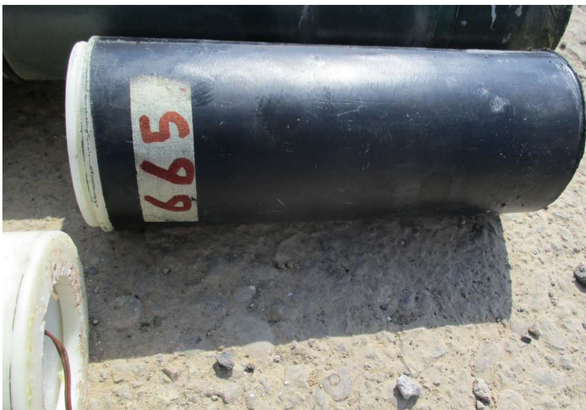
Figure 3.14 The counterweight used with IS light recoilless gun designs. This example was found with a Type 3 recoilless gun. Note the wire for the electric match protruding from the base of the expelling/propelling charge (source: Drew Prater).
