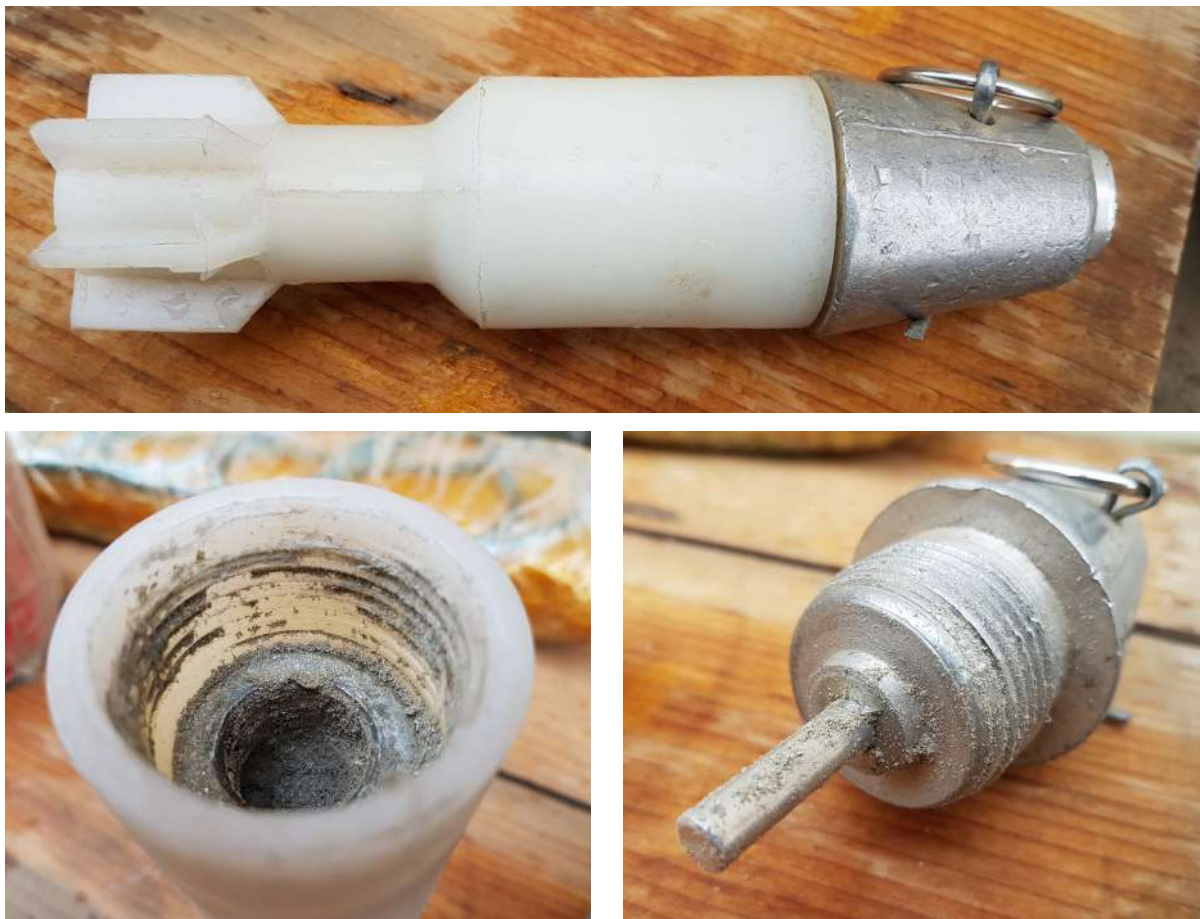
Figure 2.2 An example of one of the small craft-produced munitions developed by IS: a projected rifle grenade (fired from a cup-type launcher) and later adapted for delivery by small UAVs. Note that this munition uses an AN-A1 fill produced by IS (source: ARES/confidential).
