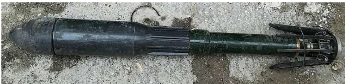
Figure 5.8 A Type 5 chemical munition. Note the flight motor taken from a PG-9 rocket-assisted munition mated to a craft-produced body (source: Drew Prater).
